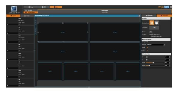
The operators' monitor layout is configured under EDIT/LIVE -> Monitoring. The layout can be in mosaic/multiviewer mode with several windows/widgets, or fullscreen mode where only one window is displayed. 12 windows/widgets are available on all LiveCore™ operator's Monitoring outputs, with the exception of the **NeXtage 08** and **NeXtage 16**, which have only 8.
