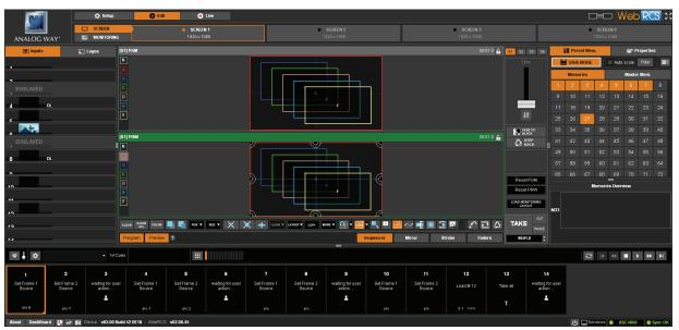
The sequencer is found at the bottom of the Edit and Live pages. Click on the **SEQUENCER** button to expand the sequencer toolbar.
