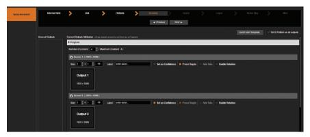
The confidence menu permits the customization of any outputs configured as confidence monitors. First of all you need to set up one of your output as a confidence output. To do that, please go under the preconfig menu, then "screens". Select one of your screens and enable the "SET AS CONFIDENCE" button. The confidence button is only available on Program screens.
