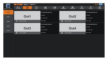
In the Output section, you can manage your output resolutions, formats, sync types, test patterns, etc...
