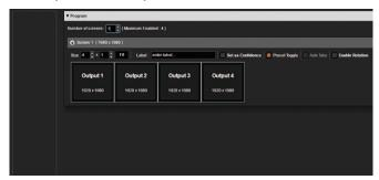
In order to simplify set up implementation, a variety of screens configuration templates are included and an id pattern can be displayed on each output.
