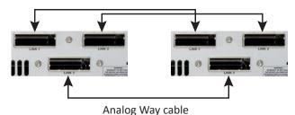
Associative Modularity mode allows for up to four units to be used as part of the same Assembly on the Vertige™ console. The Device Sync connection assists with synchronization between the various units. In Associative Modularity configuration, video information must be externally split and shared with all devices in the Assembly.
