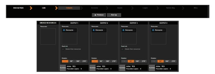
The Outputs section defines if you use any of the outputs in Dual Link or 4k modes, or if you reassign the layer resources of an output to another one. To activate a Dual Link output, drag the adjacent resources onto output #1 or #3, then check the Dual Link option box.
