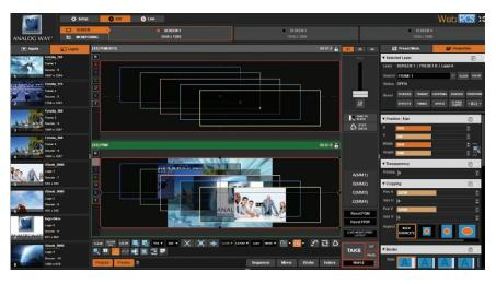
The Preview screen is now displayed into the Program screen. By default, the unit works with the **PRESET TOGGLE** mode. That means, after a **TAKE**, the Preview becomes the previous Program. While in **PRESET TOGGLE** mode, pressing TAKE repeatedly will alternate the Program screen between two different looks.
