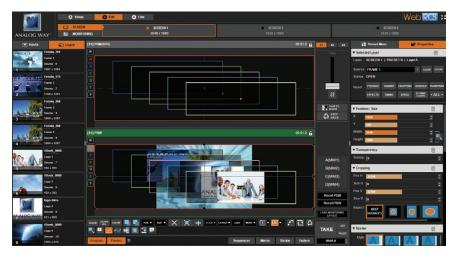
In this example, different inputs are assigned to each of the 6 layers into the Screen 1 Preview. Pressing the **TAKE** button on the bottom right side will update the Program screen based on the configuration that's been arranged in Preview.
