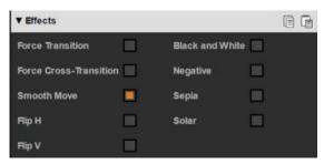
For example, disabling force transition, a PIP of camera 1 moved across the screen will move and resize to the new position. By applying Force Transition to the layer on preview which has the new position, it will force the unit to use the closing transition (ie: fade out) for the on-screen PIP of camera 1 and force the PIP that is entering from preview to use the opening transition (ie: fade in).
