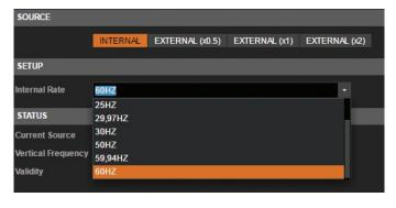
By choosing to follow one of the inputs or the framelock connector: select external and define which from plug the reference rate will be copied [EXTERNAL]
