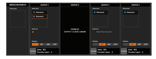
To activate an output for 4k resolutions via HDMI 1.4 (on units with the 4k hardware option), drag the adjacent resources to outputs #2 or #4 and then check the «4k» option box.
