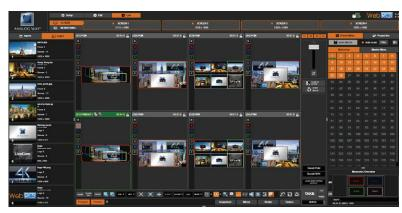
If you want to change an input into your preset into the live mode, simply use the left source ribbon and drag and drop your input into a layer.
