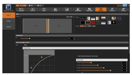
To setup an effective blend, you will first need to physically align the projected images so they are square with each other. Remember that you can adjust the number of lines and rows on the **LiveCore™** grid test pattern. to assist you.
