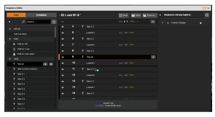
one sequence can be loaded at a time. To add a new cue to the sequence, open the Cues toolbar and select any cue from the list. The possible cues are grouped by function and include items like "Wait for X Second" or "TAKE" or "load preset " or "Set Frame slot 1 source" or "Set layer fullscreen" etc. Use the search bar at the top to help find a specific cue action.
