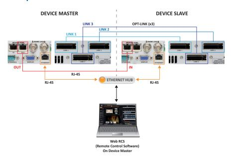
Once the two devices are wired up, ensure that all devices have unique IP addresses on the network, and that the gateway IP of all devices is set correctly. If you are not using a router on the network, set all of the gateway IP addresses to the first or last IP on the network, for example 192.168.2.1 and do not use this address for any other device.
