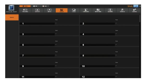
In the Library management, under the **SETUP** menu, you can find 100 empty slots that you can load one by one either with a frame or a logo that will be used later in the Edit screen. After loading, every Logo/Frame can be individually deleted by clicking on the Red Cross.
