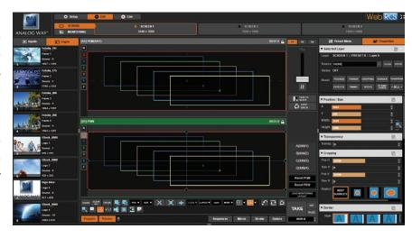
To display an input into one of the available layers A, B, C, D, E or F simply drag and drop the input from the left to the layer on the chosen screen. Remember that a layer can display an input or also logos or frames.
