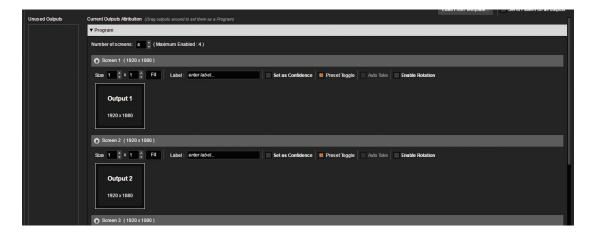
Drag and drop the available outputs into the desired screen destination. By default, your screens will mapped Output #1 = Screen #1, Output #2 = Screen #2 etc. You can change this order and put for example the Output #3 into the Screen #1
