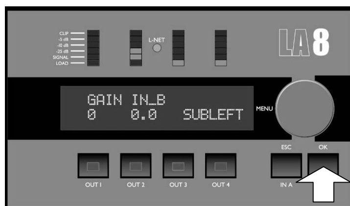
Figure 21: Controller’s group indication
