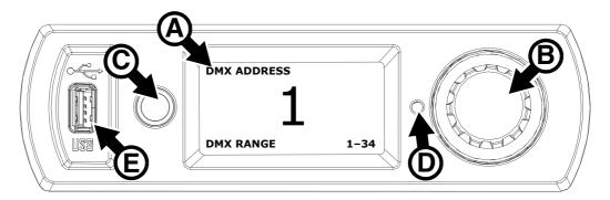
Figure 2: Display and control panel
