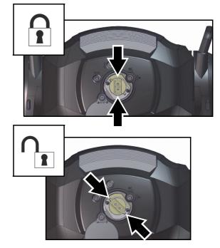
Figure 9: Lamp lock / unlock
