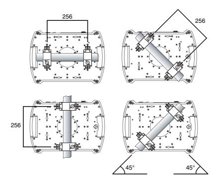
Figure 2: Clamp bracket positions
