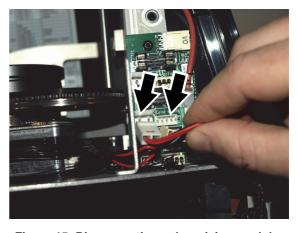
Figure 15: Disconnecting color mixing module
