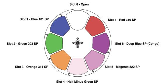
Figure 1: Color wheel (seen from lamp side)
