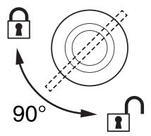
Figure 5: Locking 1/4-turn fasteners
