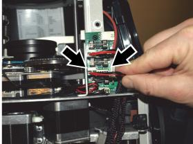
Figure 20: Connecting the IBD module
