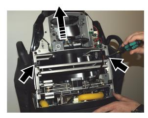
Figure 17: Releasing the aperture plate module
