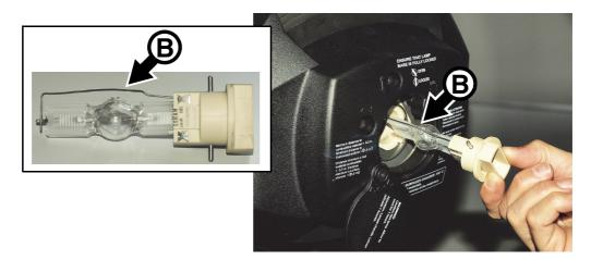
Figure 10: Lamp removal / refitting
