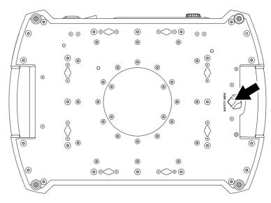
Figure 6: Safety cable attachment point
