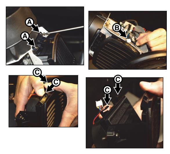
Figure 13: Head air filter removal
