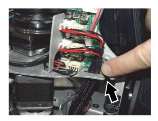
Figure 21: Module wireset routing
