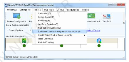
Note: After entering the **Configuration File of Controller Cabinet Import** window, NovaLCT will automatically read the configuration files already existed in the MCTRL R5. Users can change the names and orders of these files or delete them.
