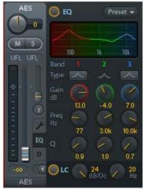
**Lo Cut.** Activated by the button Lo Cut. The slope of the high-pass filter is adjustable between 6, 12, 18 and 24 dB per octave. The cut-off point (-3 dB) is adjustable between 20 Hz and 500 Hz.
