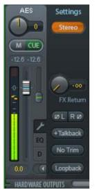
Another difference to the input and playback channels is the **Cue** button instead of Solo. A click on Cue sends the respective Hardware Output's audio to the **Main** Out, or any of the Phones outputs (option *Assign / Cue to* in the Control Room section). With this any hardware output can be controlled and listened to through the monitoring output very conveniently.
